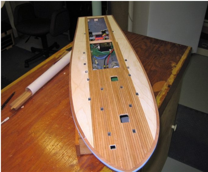
Applying cherry planking and "Dead Lights" to the sub deck.
